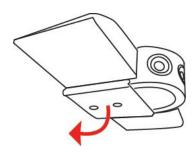
· Place camera on top of a flat-panel monitor and adjust to your preferred position.
