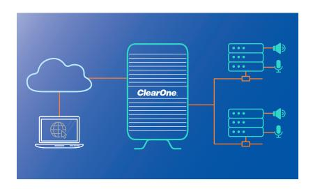
CONVERGENCE InSite Server is network hardware that enables bi-directional communications between Cloud AV Manager or Enterprise AV Manager and on-site ClearOne Pro Audio devices.
